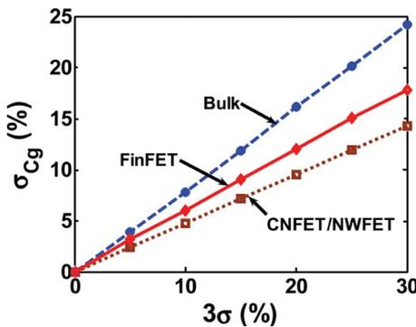
Fig. 9. Overall gate capacitance  $C_g$  sensitivity to all parameter variations. The approximate linear response demonstrates the dominance of the  $W$  variation.  $C_{fr}$  was added to the FinFET device based on [12] because the original model had zero fringe capacitance.
