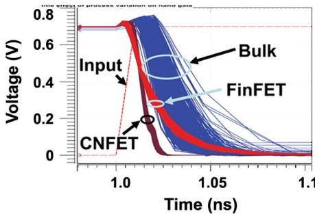
Fig. 10. Delay variation of a two-input NAND with an inverter load at the 32 nm technology node ( $V_{dd} = 0.7$  V and  $3\sigma = 15\%$ ).  $C_{fr}$  of the FinFET device was modified based on [12]. The NWFET result was similar to that of the CNFET but is not shown due to clarity.
