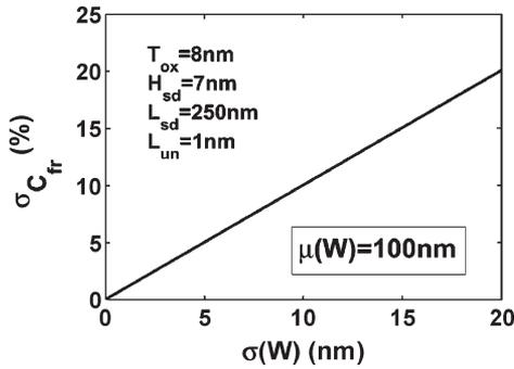
Fig. 8.  $C_{fr}$  sensitivity to the  $W$  variation. Note that  $\sigma_{C_{fr}}$  approximately linearly changes with the  $W$  variation. The linear change is due to the linear dependence of  $C_{fr}$  on  $W$ .
