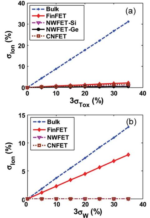
Fig. 4. Sensitivity of  $I_{on}$  of an NFET to (a)  $T_{ox}$  and (b)  $W$  variations.  $I_{on}$  of a FinFET device is less sensitive to the  $W$  variation than a bulk device due to less narrow-width effect; whereas, it is not sensitive in the NWFET/CNFET devices, as explained earlier (see Fig. 1).
