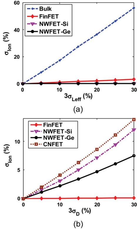
Fig. 5.  $I_{on}$  sensitivity to (a) the  $L_{eff}$  variation and (b) diameter of nanotube/nanowire and body thickness  $T_{si}$  variations of a FinFET. Note that the  $L_{eff}$  variation is attributed to both the wire orientation variation and the lithography variation.
