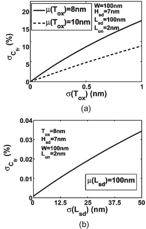
Fig. 7. Sensitivity of NWFET/CNFET fringe capacitance to  $T_{ox}$  and source/drain length variations. Due to logarithmic dependence,  $\sigma_{C_{fr}}/\sigma_{T_{ox}}$  is less than 1. The effects of gate thickness  $T_g$  and underlap  $L_{un}$  variations are similar to  $L_{sd}$  and  $T_{ox}$  variations, respectively, due to geometrical symmetry and, hence, are not shown here.
